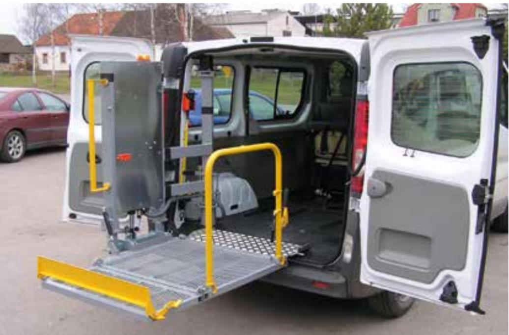
The interior column lift DH-VZH is designed to suit a wide range of Multi Passenger Vehicles, minibuses, coaches, trains, ...
