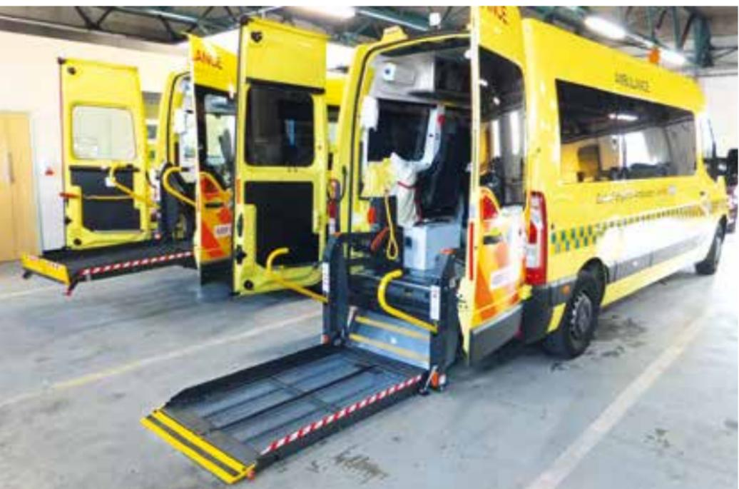
The reinforced linear 2-arm lift offers 500 kg lift capacity and fulfills the most demanding requirements of the passenger transport sector. The platform depth can be extended to 1600 mm to **load and unload hospital stretchers**. The platform width can be increased to 920 mm to suit **bariatric applications**, both wheelchairs and stretchers.
