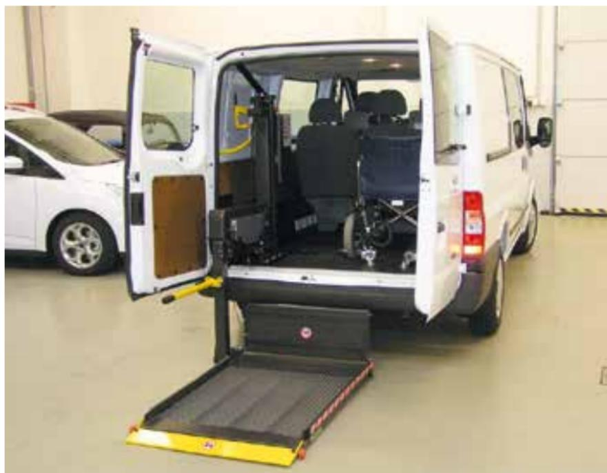
The DH-PH1 is a **linear 1-arm lift**, suitable for mounting inside the rear or side doors of a wide range of Multi Passenger Vehicles, minibuses and ambulance vehicles.
