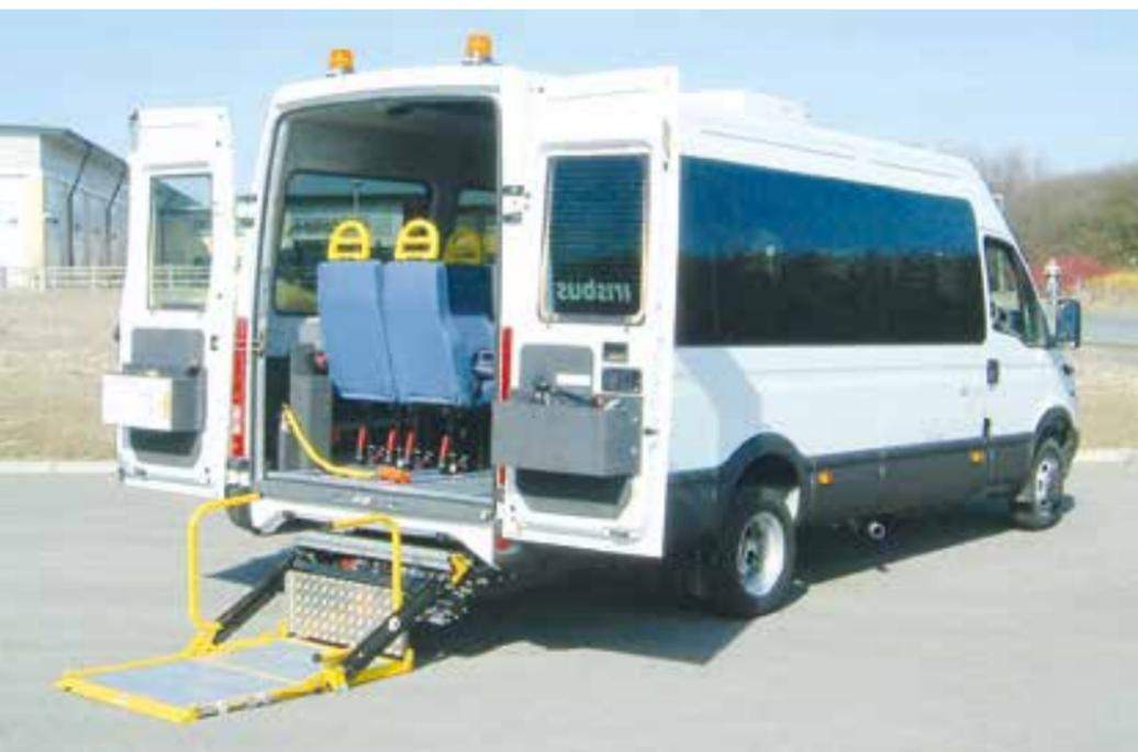
The passenger lift DH-CH001 stows neatly in a sealed cassette box under the loading floor of the vehicle. This solution keeps the **access through the rear doors free** and **occupies no space inside the vehicle**.
