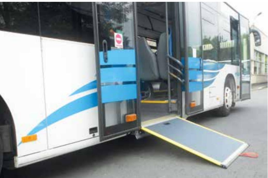
The access ramps DH-BRM... are designed to assist wheelchair passengers, parents with a baby buggy, or passengers with an otherwise impaired mobility to enter or exit the bus safely and comfortably.
