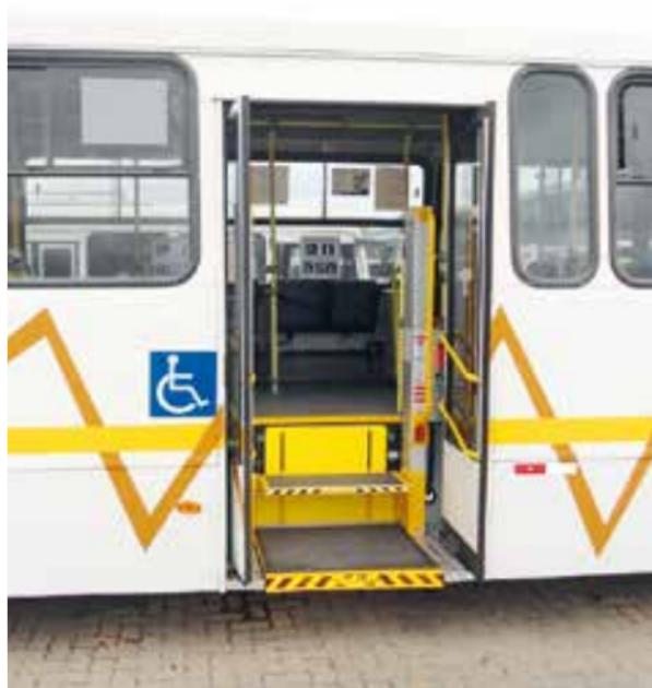
The **DH-TV 300 kg** is specially designed for **urban buses**, to assist wheelchair passengers to embark and disembark the vehicle in a comfortable and safe manner.
