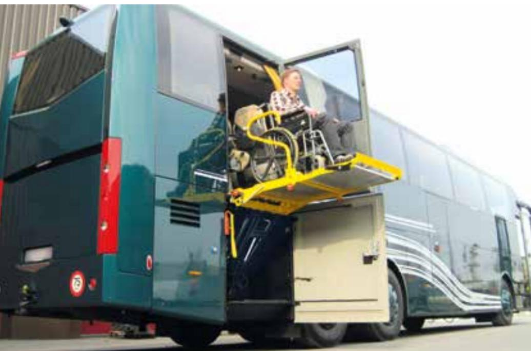
The **fold-away** lift DH-RB is specially designed for coaches, to help wheelchair passengers to embark and disembark the vehicle in a comfortable and safe manner.
