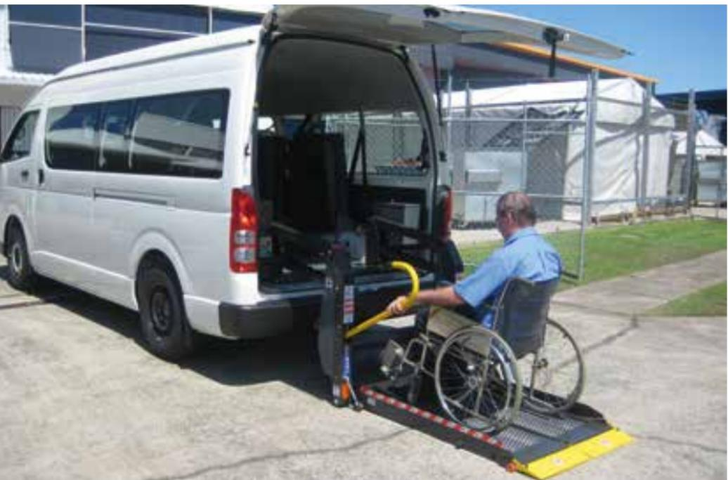
The DH-PH2 belongs to a new generation (2010-...) of **fully automatic linear passenger lifts**. It is suitable for mounting inside the rear doors of a wide range of Multi Passenger Vehicles, minibuses and ambulance vehicles.
