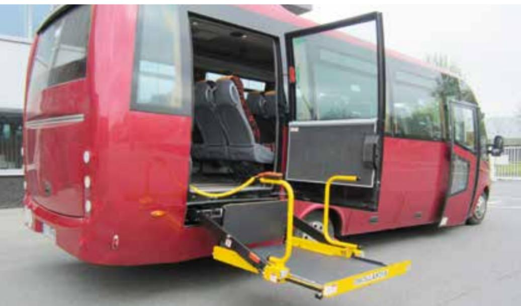
In comparison to the DH-CH100...103, the DH-CH002 and -CH003 are equipped with **extensible platforms**, significantly **reducing the required fitting space** under or inside the vehicle.
