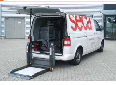
The DH-P2 is a fully automatic linear lift, suitable for mounting **inside the cargo space** of the vehicle. It can be mounted at the rear doors or at the side doors of a wide range of Multi Passenger vehicles and vans.
