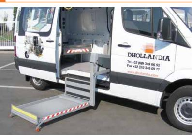
The DH-P1 is a **linear 1-arm lift**, suitable for mounting inside the rear or side doors of a wide range of Multi Passenger Vehicles and vans.
