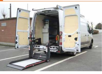
The DH-P2.07 is the **heavy-duty execution** of the **DHOLLANDIA** range of internally mounted lifts. It offers:
