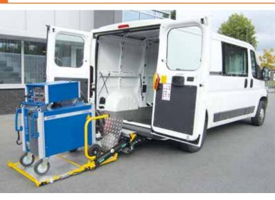
The cassette lift DH-C001 stows neatly in a sealed cassette box under the loading floor of the vehicle. This solution keeps the **access through the rear doors free** and **occupies no space inside the vehicle**.
