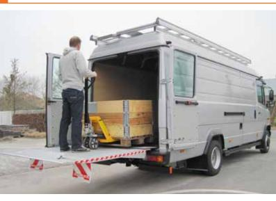
The DH-LC.15 offers 1500 kg lift capacity for the **higher capacity factory built panel vans** from 4.5 up to 7.5T GVW (e.g. Mercedes Vario, lveco Daily,...).
