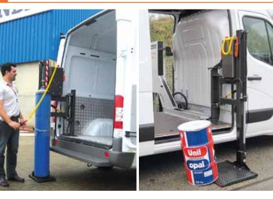
The DH-VZG is a safe and easy-to-use compact interior lift, designed to handle **small loads** (parcels, boxes, barrels, small machinery,...).
