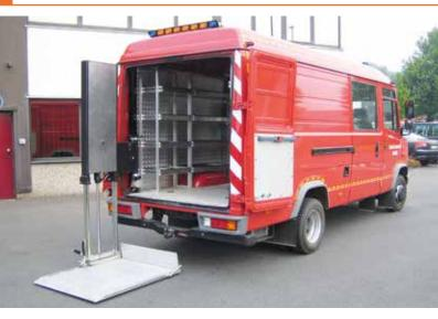
The interior column lift DH-VZ is designed to suit a wide range of Multi Passenger Vehicles, vans, and even larger commercial vehicles.
