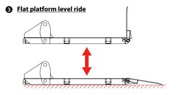
The platform remains level during the full lifting / lowering cycles. The rear end of the platform can be a fixed leading edge, or hinged ramps which adjust more easily to uneven surfaces.
