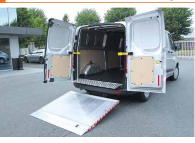
The DH-LSP was the first external lift ever in the tail lift industry, engineered to suit factory built panel vans. DHOLLANDIA still continues to lead the innovations in this field today. The intelligent shape of the lift arms eliminates the need to cut in the vehicle chassis or rear floor cross member, and maximises the ground clearance under the lift.
