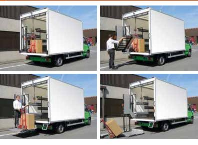
In its travel position, the interior lift **DH-VZS** is stowed against the side of the body and offers the driver **quick and free access** through the vehicle doors. Upon use, the platform is simply pulled out and opened by hand. As the platform slides straight towards the door exit, the floor space beside it can be fully occupied (as opposed to the DH-VZ.03). A wander lead with spiral cable is used to operate the platform up and down.
