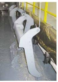
**HOT-DIP ZINC PLATING** is based on the metallurgic bond between the steel parts and zinc, melted at 460 °C. The zinc-iron alloys formed in this way, offer a number of clear advantages:
