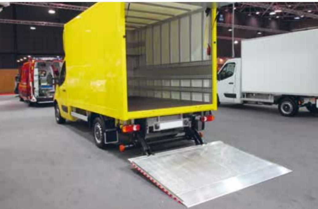
The new DH-LE is a **light-weight 2-cylinder lift**, at the entry level of DHOLLANDIA's range of cantilever lifts. Thanks to its compact lift frame and short lift arms, it ideally suits light commercial vehicles with **very short overhang**.
