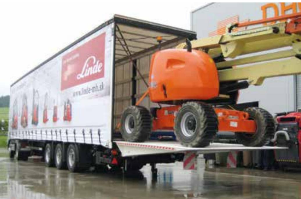
The heavy duty lift DH-LSU.90 is designed for **extreme lift capacities from 7,500 to 9,000 kg** and is mainly used for the transport of heavy machinery, forklifts, agricultural tractors etc...
