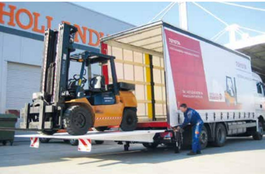
The heavy duty lift DH-LSU.60 is designed for **extreme lift capacities from 4,000 to 6,000 kg** and is mainly used for the transport of heavy machinery, forklifts, agricultural tractors etc...
