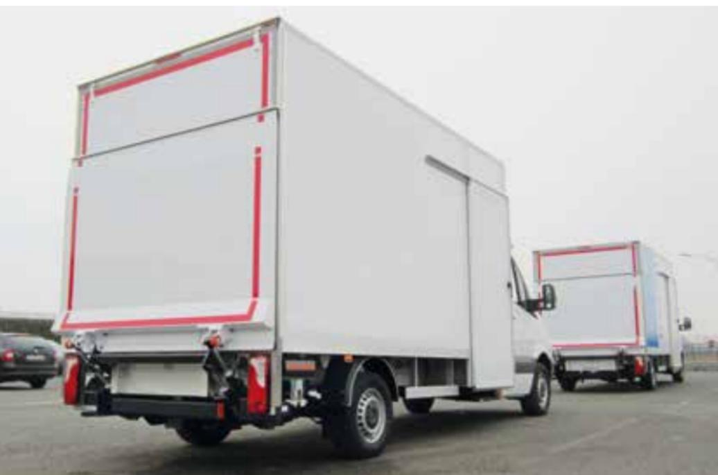
The DH-LSP4 is equipped with a compact lift frame and **very short lift arms**.
