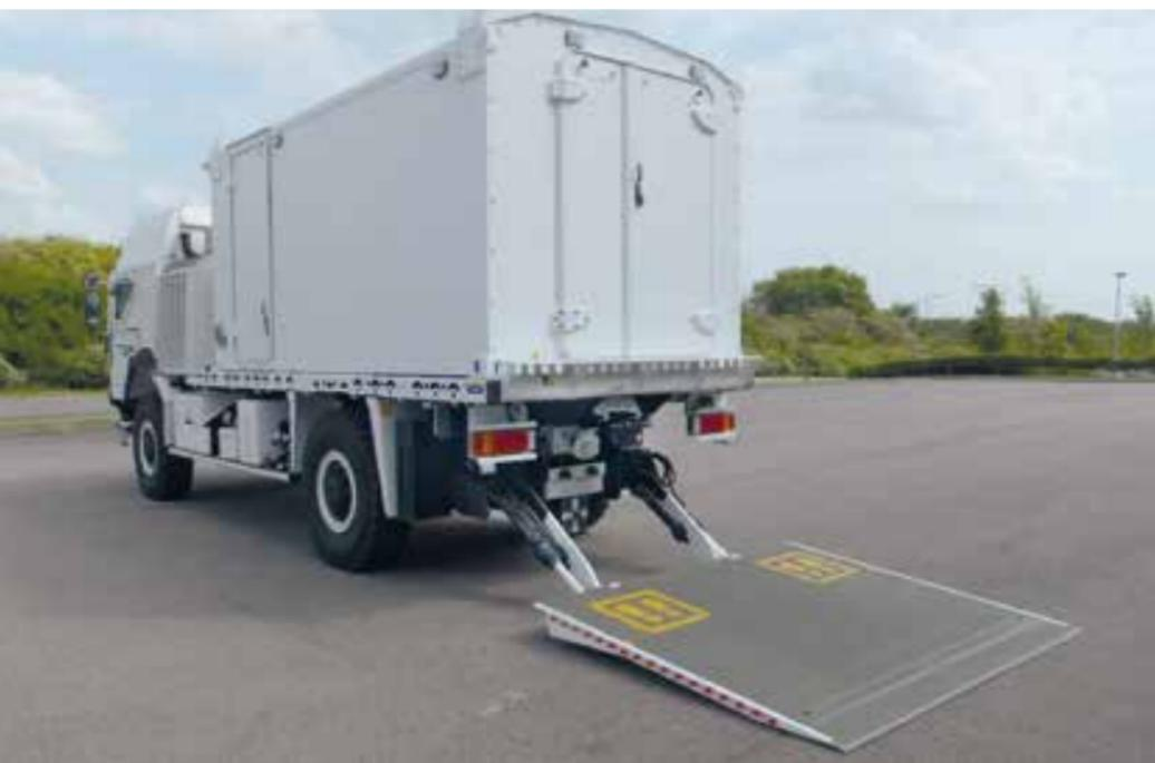
The DH-LMP.20 is equipped with a **compact lift frame**, that requires 100 mm less overhang than the standard model DH-LM.20. It is specially adapted to suit trucks, trailers and semi-trailers with a **very short overhang** behind the rear axle or the spring hangers on the vehicle chassis (e.g. military trucks, city-trailers with rear steering axle,...)
