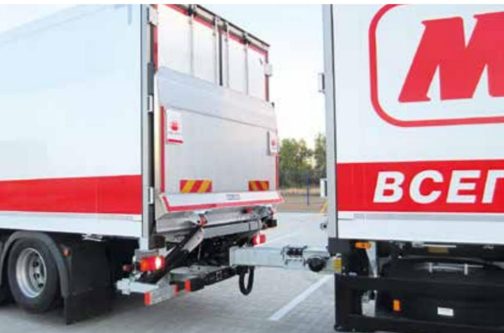
The DH-LM.15 was launched in 2012 as missing link between the 1000 and 2000 kg capacity lifts. Since then, it has become extremely popular as **ideal weight saving lift for medium capacity trucks** of 7,5T to 12T GVW.
