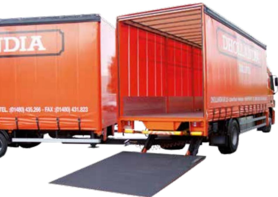
The **DH-LV** is designed for **trucks with a draw bar coupling** mounted below the vehicle chassis, to function in combination with a **centre-axle trailer**.
