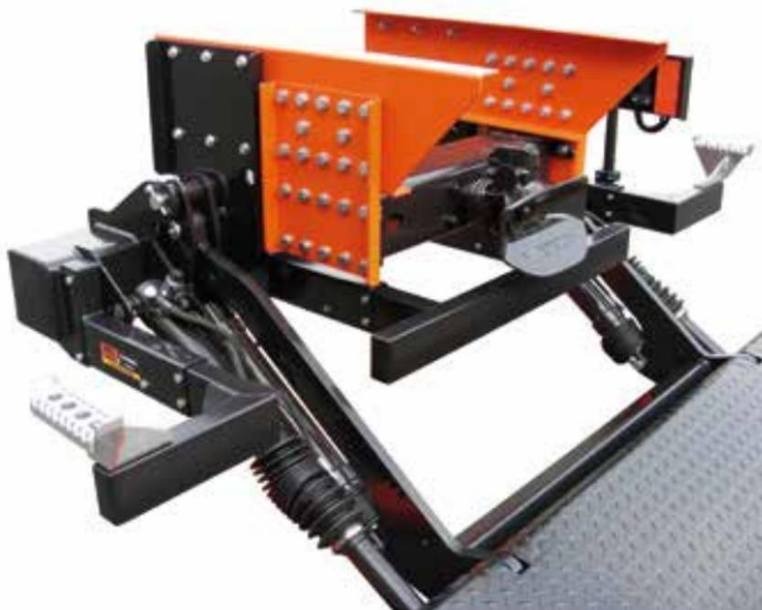
The DH-LM.30 with option OAU001 foresees in a **3-piece bumper bar that is adjustable in height and in length**. Hence it is suitable for trailer couplings mounted under the truck chassis, completely at the rear of the chassis beams. This configuration is most common in Scandinavia / Sweden. OAU001 is equipped with double acting tilt cylinders.
