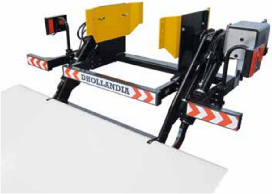
**OAU002** is a special execution of the DH-LV.40, specially adapted for trailer couplings mounted under the truck chassis, but approx. 1 m in front of the rear of the vehicle body. This configuration is popular in Finland. The (yellow) mounting plates of the lift wrap around the mounting plates of the trailer coupling.
