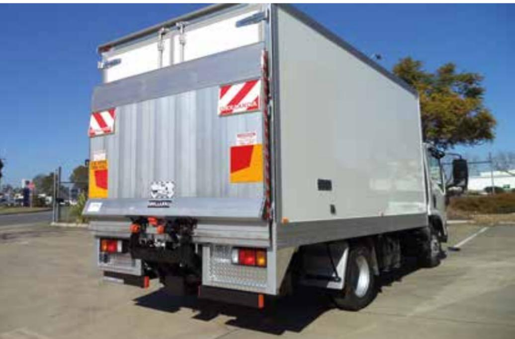
The **2-cylinder** DH-LC is at the entry level of DHOLLANDIA's range of cantilever lifts. Thanks to its intrinsic simplicity, its low maintenance cost and its attractive pricing, this compact lift is ideal to equip **rental vehicles** and **light-duty commercial vehicles**.
