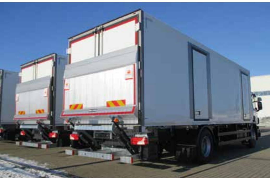
The DH-LM.20 is an **extremely versatile medium capacity lift**, suitable for commercial trucks above 7.5T GVW, trailers and semi-trailers.
